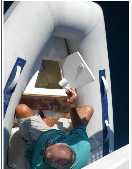
Paint to protect the epoxy
